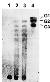
Fig. 4. TLC of the hydrolysis products of laminarin by tomato \beta -1,3-glucanase. Lanes 1, 2 and 3, hydrolysis for 0, 1 and 3 h, respectively; lane 4, standards (G1, glucose; G2, laminaribiose; G3, laminaritriose).
